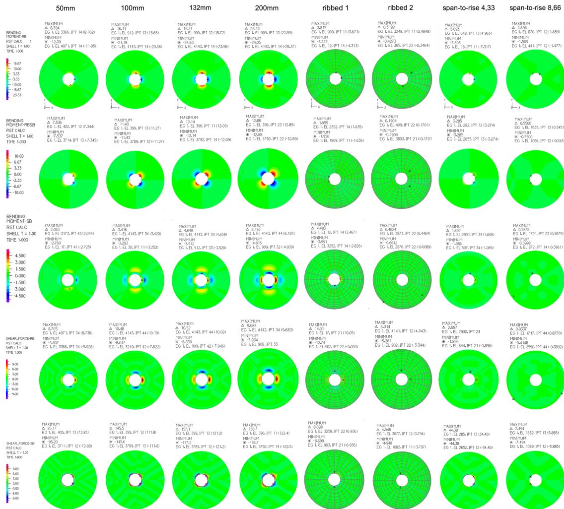
Figure 4.9 - Distributions of M_{RB} \equiv M_{\varphi\varphi} , M_{SB} \equiv M_{\theta\theta} , M_{RBSB} \equiv M_{\theta\varphi} [kNm/m] and Q_{RB} \equiv Q_{\varphi} , Q_{SB} \equiv Q_{\theta} [kN] for ULS (wind as v.l.).
